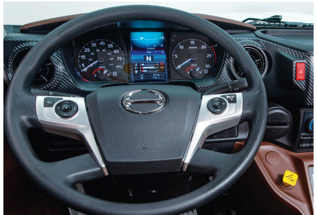
The LED driver display allows the driver to scroll through a series of menus to view current and historical fuel economy as well as engine parameters.
