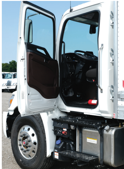
The driver's door opens a full 80 degrees, allowing easy cab entry and exit. The climb up is made safer with a pair of well-placed grab handles.
